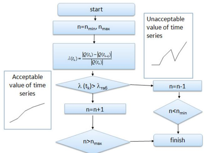
**Fig. 5. Regularization algorithm.**
